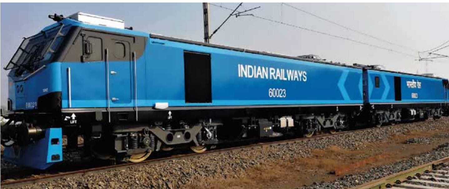
8 Ø1250 mm locomotive wheel Alstom electric double-section locomotives of 12,000 HP, Indian Railways
