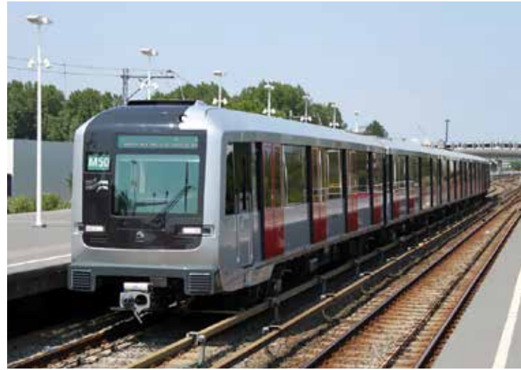
Ø840 mm wheel Alstom M5 Metropolis metro cars, The Amsterdam Metro, the Netherland
