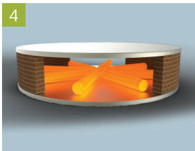
4 Heating of billet in rotary furnace
