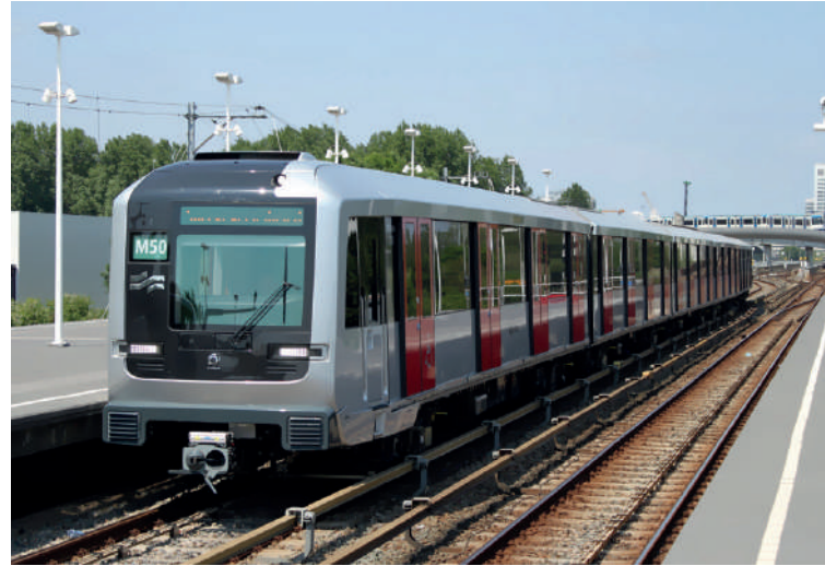
Ø840 mm wheel Alstom M5 Metropolis metro cars, The Amsterdam Metro, the Netherlands
