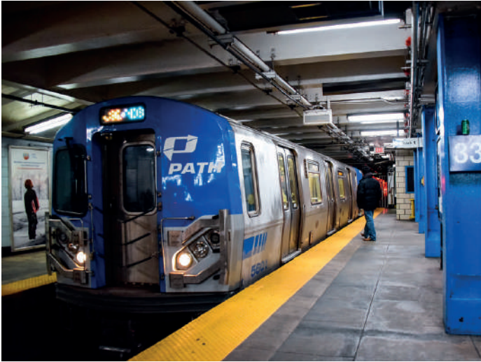
Ø870 mm wheel Kawasaki PA-5 metro cars, PATH (New York – New Jersey), the USA
