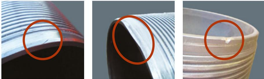
Poor alignment and make-up cause galling. (connection should be rejected)
