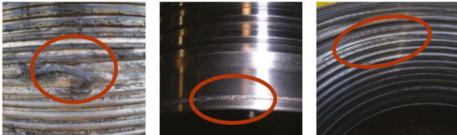
Improper storage causes rust, corrosion or pitting. (connection should be rejected)
