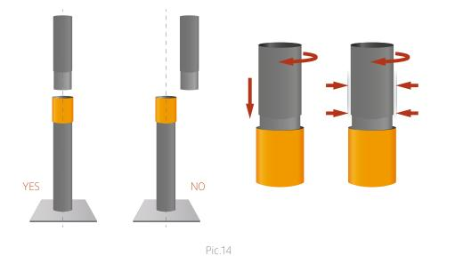
• Be careful when stabbing the pin end into the box, do not damage seal area. To minimize this risk, over the box connection use a plastic or rubber stabbing guide (see pic. 15). Control stabbing process, lower pin into box gradually. If a fault occurs when stabbing, check alignment and slowly rotate the pipe in reverse until the threads drop. Do not roll pin into box.
