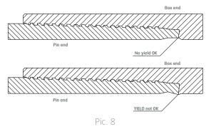
No step at the shoulder, check weight of installed coupling to the pipe body.
