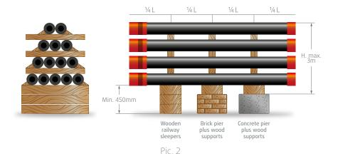
• Pipes of the same type OD, wall thickness, group strength should be placed at the same rack. Do not mix pipes of different grades when storing, as this makes it more difficult to locate them for pre-running inspections and can lead to grade mixing in the well.
