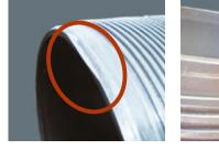
Poor alignment and make-up cause galling. (connection should be rejected)
