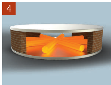
4 Heating of billet in rotary furnace
